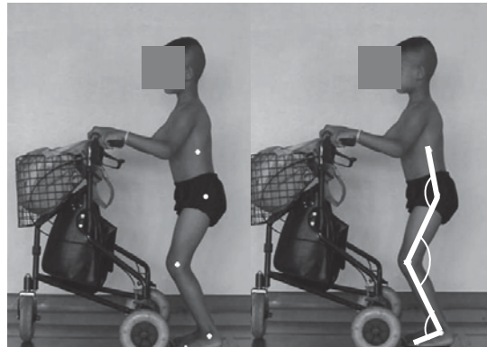
Figure 11 Position of participant for assessment of hip, knee and ankle joints angle during standing
