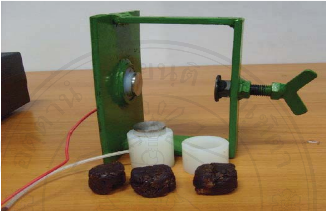
Figure 3.5 Proposed dried longan aril-based capacitor
