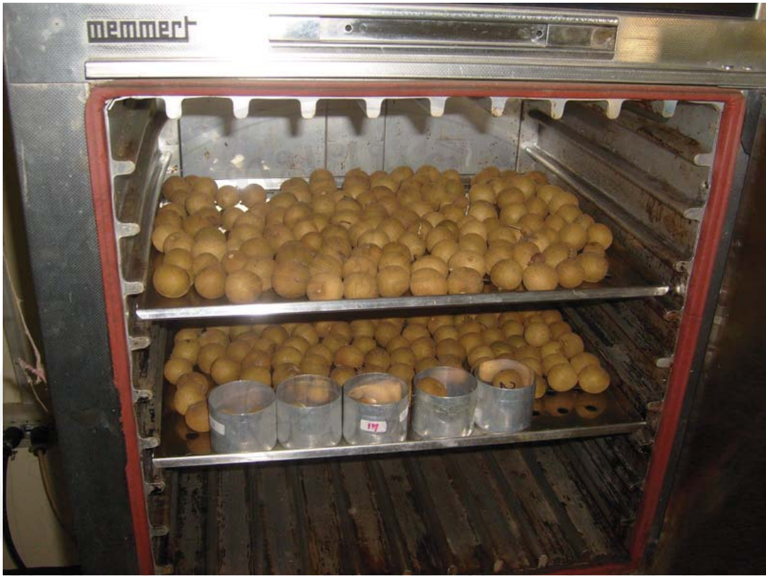
Figure 3.12 Longan drying process: moisture content was estimated by hot air oven
