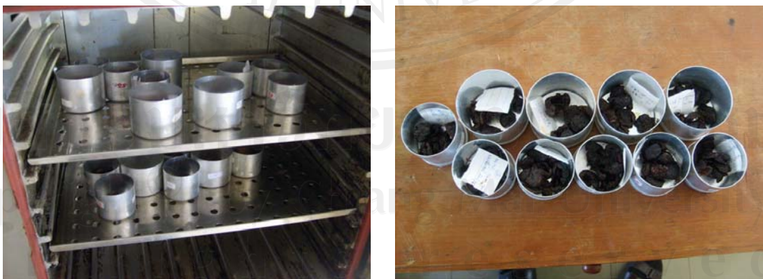
Figure 3.15 Actual moisture content dried at 70 °C under vacuum for about 8 hours or until their weights are constants.
